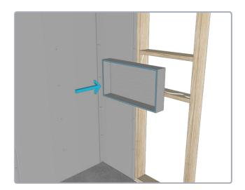
**4.** Ensure the niche is aligned with precision, and double-check that it is completely level. If needed, secure it in place with screws.
