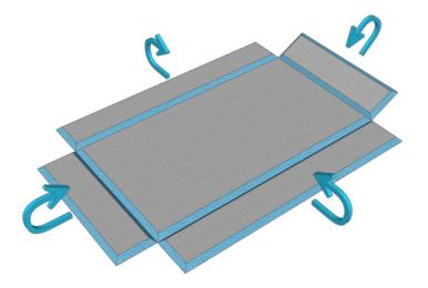
**3.** Spread a continuous bead of a non-solvent based adhesive along the surrounding framework and fit it to the wall cavity.
